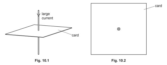
There is a pattern of magnetic field lines around the wire due to the current in the wire.
