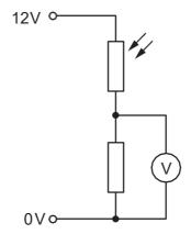
The light falling on the light-dependent resistor (LDR) increases in brightness.
