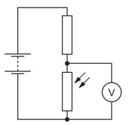
A bright lamp shines light onto the LDR. The lamp is then switched off and this causes the voltmeter reading to change.
