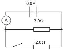
The switch is open, and the ammeter reads 2.0 A.
