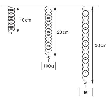
The extension of the spring is directly proportional to the mass hung on it.
