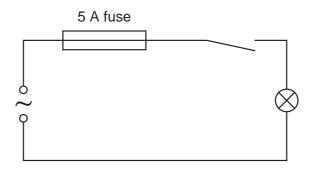
The fuse has blown and stopped the current.
