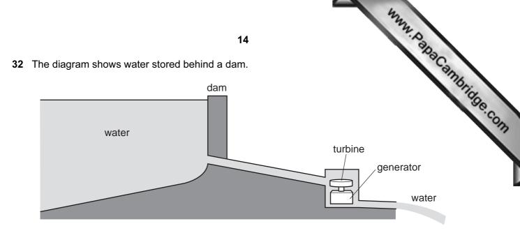
The water flows to a turbine and turns a generator.
