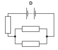
39 In the circuit below, one of the lamps breaks, causing all the other lamps to go out.
