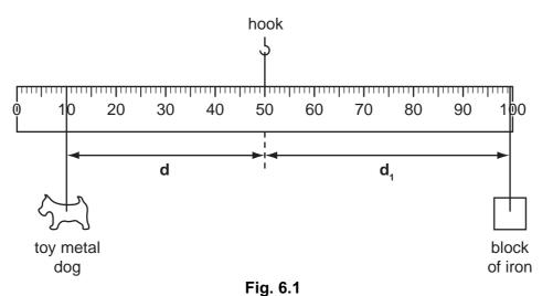
The dog is moved to another position and the block is moved until the rule balances again. This is repeated several times and the results recorded in Table 6.1.
