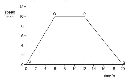
Between which points on the graph is the acceleration zero?
