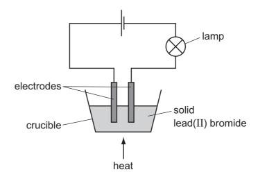
The crucible needs to be heated for the lamp to give out light.
