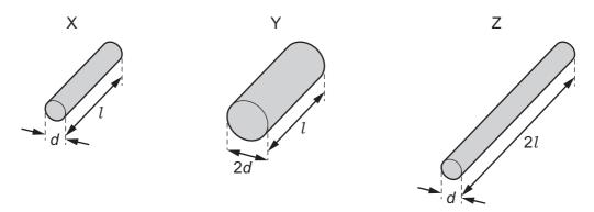
What is the order of the wires when they are placed in order of increasing resistance, least resistance first?
