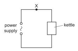
If too much current flows, a component connected at X automatically disconnects the power supply.
