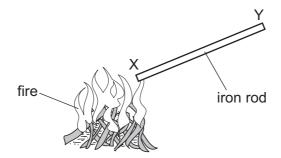
The other end Y of the rod becomes warm by thermal conduction through the rod.
