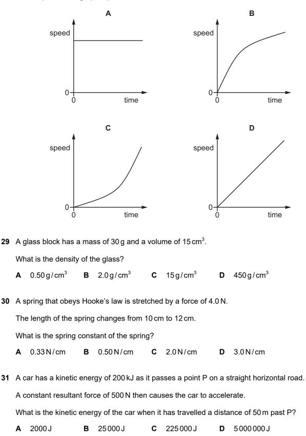
28 Which speed-time graph represents motion for which the acceleration is constant but not zero?
