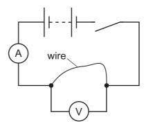
When the switch is closed, the ammeter reads 2.0 A and the voltmeter reads 10 V.
