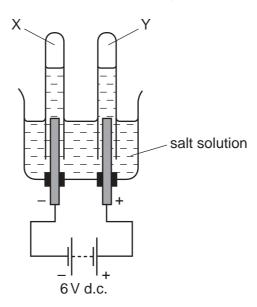
One of the gases explodes when tested with a burning splint and the other turns moist Universal Indicator paper red then white.
