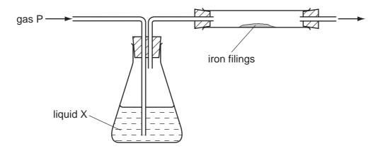
Which gas and liquid cause the iron to rust?
