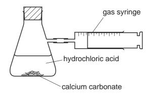
The time to collect 50 cm<sup>3</sup> of gas is measured.
