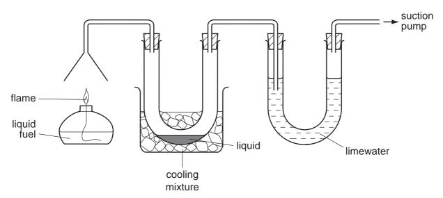
Which substances is the apparatus testing for?
