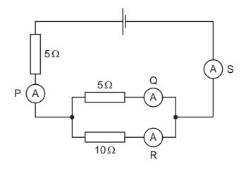
Which statement about the readings on the ammeters is correct?
