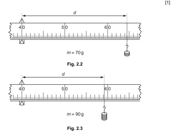
(iii) Calculate, to three decimal places, the values of  $\frac{1}{m}$  for the masses 70 g and 90 g. Record these values in Table 2.1.
