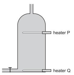
When only heater Q is switched on, it takes a long time to heat the tank of water to the required temperature of 60 °C.
