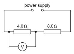
The reading on the voltmeter connected across the  $4.0\,\Omega$  resistor is  $2.0\,V$ .
