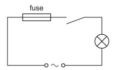
When the switch is closed the fuse blows and stops the current.
