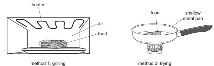
How does thermal energy pass through the air to reach the food in method 1 and how does thermal energy pass through the bottom of the metal pan in method 2?
