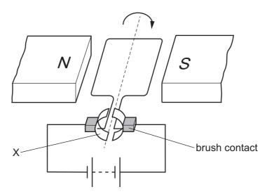
What is the name of part X and how does it help the motor to work?
