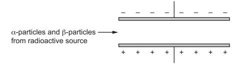
In which directions are the particles deflected as they pass between the plates and which particles are deflected more?
