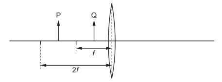
The object is moved to position Q. The image produced is now virtual.
