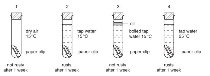
Which two experiments can be used to show that air is needed for iron to rust?
