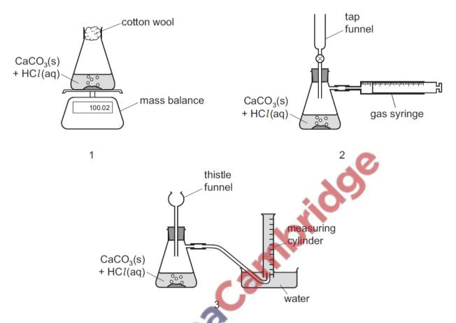
Which sets of apparatus are suitable, together with a stop-watch, for following the rate of this reaction?
