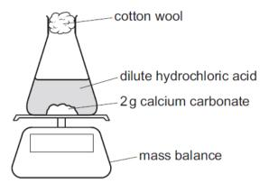
In experiment 1, the calcium carbonate is powdered and an excess of hydrochloric acid is used.
