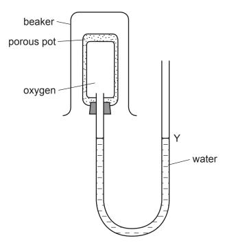
Which gas, when present in the beaker over the porous pot, will cause the water level at Y to rise?
