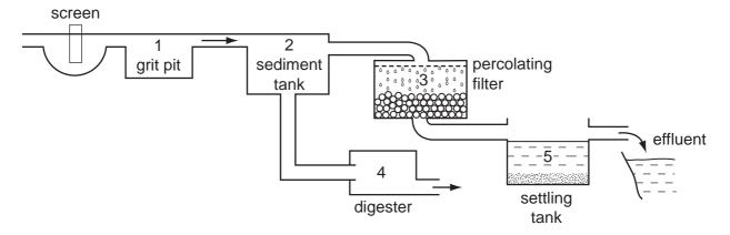
In which parts do aerobic and anaerobic bacteria become most active to help to digest sewage?
