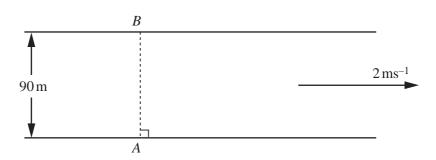
The diagram shows a river 90 m wide, flowing at  $2 \,\mathrm{ms^{-1}}$  between parallel banks. A ferry travels in a straight line from a point A to a point B directly opposite A. Given that the ferry takes exactly one minute to cross the river, find
