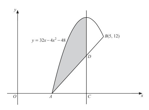
The diagram shows part of the curve  $y = 32x - 4x^2 - 48$  and the line *AB*. The curve and the line *AB* meet the *x*-axis at *A* and meet again at the point *B*(5, 12). The line *CD* extended is parallel to the *y*-axis and passes through the maximum point of the curve. Find the area of the shaded region. [9]
