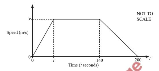
(a) The deceleration of the car between t = 140 and t = 200 is  $0.2 \,\mathrm{m/s}^2$
