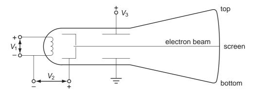
Which change in voltage results in the position of the spot on the screen moving towards the top?
