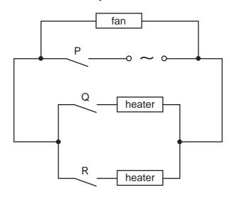
The fan has a power rating of 0.1 kW and the heaters each have a rating of 0.4 kW. The cost of electricity is 8 cents/kW h.
