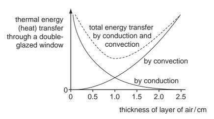
Which thickness of air produces the smallest energy transfer, and why?
