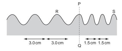
The wave has a speed of 12 cm/s at R.
