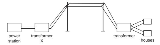
How does transformer X affect the voltage and the current from the power station?
