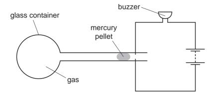
The mercury pellet moves and completes the circuit.
