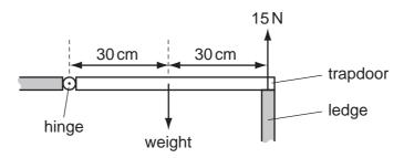
When the trapdoor is closed, the ledge exerts an upward force of 15 N on the trapdoor. The gravitational field strength is 10 N/kg.
