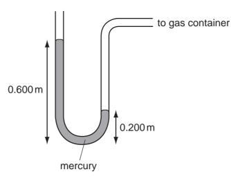
The density of mercury is  $13600 \text{ kg/m}^3$ . The gravitational field strength g is 10 N/kg.
