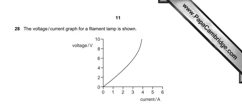
The voltage across the lamp increases. What happens to the temperature of the lamp and the resistance of the lamp?
