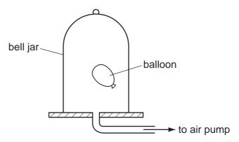
The air pump is switched on and air is removed from the bell jar.
