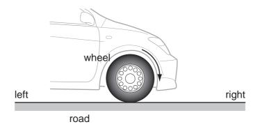
What are the directions of the frictional forces on the wheel of the car and on the road?
