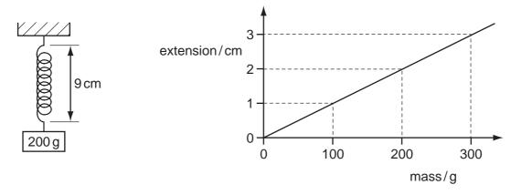
The 200 g mass is replaced with a 100 g mass. What is the new length of the spring?
