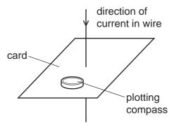
A plotting compass is placed on the card.
