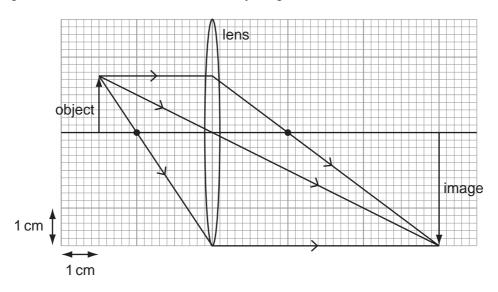
What is the linear magnification produced by the lens?
