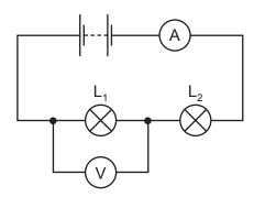
A voltmeter measures the potential difference across the lamp L<sub>1</sub>.
