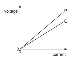
The wires are made from the same material and have equal lengths.
