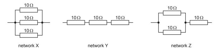
What is the order of resistance of the networks going from the smallest total resistance to the largest total resistance?
