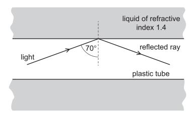
What describes the values of the critical angle in the plastic and the refractive index of the plastic?
