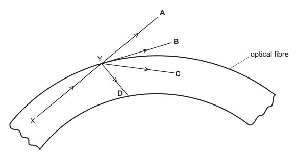
A ray of light in glass is incident on the surface at an angle *c*. The angle *c* is the critical angle. Which diagram shows what happens to the light?
