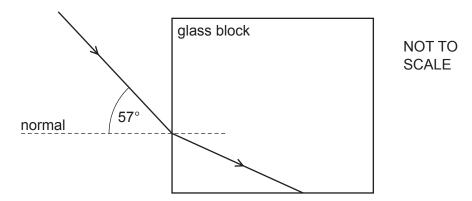
What is the angle of refraction in the glass and what is the critical angle?
