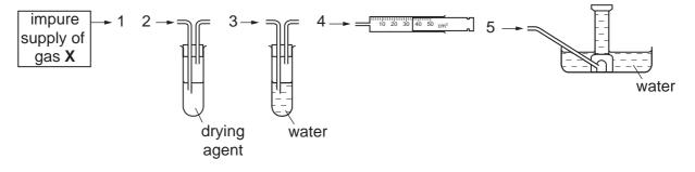
In which order should the pieces of apparatus be joined together to collect a pure, dry sample of **X**?
