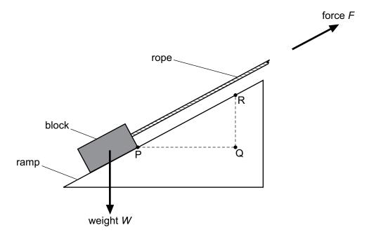
The block has weight W and the rope is pulled with force F.
