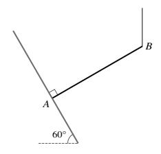
The rod rests with A on a rough plane that makes an angle of  $60^{\circ}$  to the horizontal. A string is attached to B and the rod is in equilibrium in the vertical plane containing the line of greatest slope of the plane, with the string vertical and AB perpendicular to the plane (see diagram). Find the magnitude of the frictional force at A and the tension in the string. [5]
