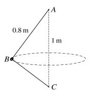
A light inextensible string of length 1.4 m has its ends attached to two points A and C, where A is 1 m vertically above C. A smooth bead B of mass 0.2 kg is threaded on the string and rotates in a horizontal circle with the string taut. The distance BA is 0.8 m (see diagram). Find
