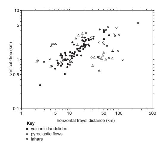
The vertical drop and horizontal travel distance of three volcanic mass movement processes
