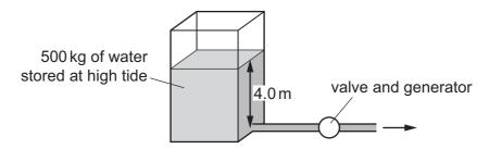
At high tide 500 kg of water is stored to a height of 4.0 m. When the valve is opened the container empties in 5.0 s and the generator operates with an efficiency of 40%.
