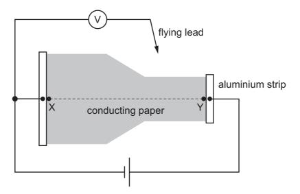
The flying lead of the voltmeter is placed in contact with the conducting surface at X and the reading noted. This is repeated for a large number of points along the line XY, ending at point Y.
