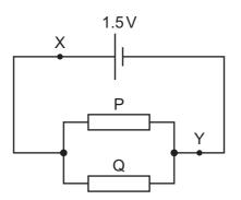
The resistors have different values of resistance. The cell has an electromotive force of 1.5 V. It has negligible internal resistance.
