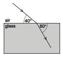
The angle between the ray and the edge of the glass block is 40° in the air and 60° in the glass.
