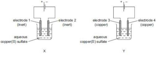
On which electrodes is solid metal deposited?
