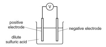
The voltages produced by different combinations of metal electrodes are shown in the table below. The more reactive metal is always the negative electrode.
