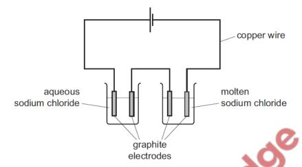
Which substance in the diagram has both positive ions and mobile electrons?
