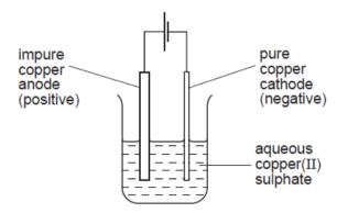
The loss in mass of the anode (positive electrode) is 50 g and the gain in mass of the cathode (negative electrode) is 45 g.
