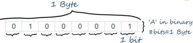
Its value is usually held in memory as an electrical charge stored in a capacitor. Modern memory chips contain millions of these tiny capacitors, each of which is capable of storing exactly one bit of information. A single bit can have one of two values at any given time
