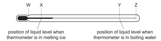
The scientist marks a scale on the thermometer that gives the temperature in degrees Celsius (°C).
