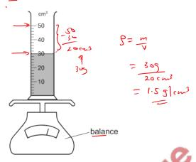
Some more of the liquid is added until the liquid level reaches the 50 cm3 mark
