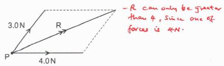
The angle between the 3.0 N force and the 4.0 N force can be any value from 0° to 90°.
