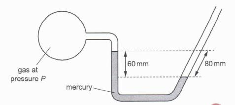
Atmospheric pressure on its own supports a column of mercury of height 756 mm.
