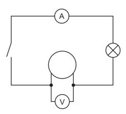
(ignore orange) to include ammeter in series and voltmeter in parallel, (allow two lamps OR two switches) correct symbols ;; (4 correct = 2 marks, 3 correct = 1 mark) no gaps or short circuits ;
