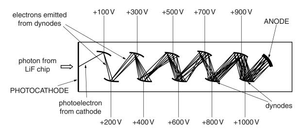
Fig. 3: schematic diagram of a photomultiplier tube
