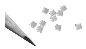
Fig. 2: some LiF chips as used in TLD, with a pencil tip for scale.
