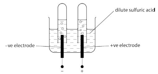
Hydrogen is made at the negative electrode.
